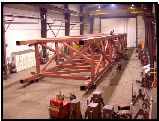
Tube Structure for USAF Hanger
